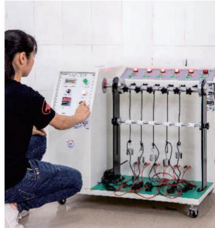
摇摆测试 Swing testing
